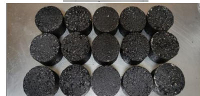
Fig. 2. Production of asphalt concrete samples
